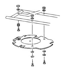
Mount the low voltage camera on the mounting plate.
