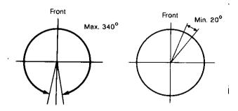
With both limit stops, pan to both stop positions and recheck for exact positioning of limit stops. Tighten both stops securely.
